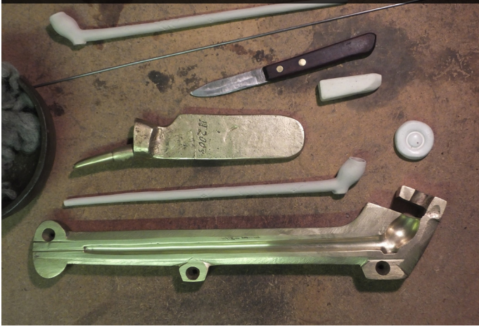
3. Freshly moulded pipes
